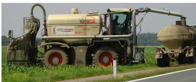
Figure 6.3 Vehicles for application of digestate as fertiliser, using dragging hoses (AGRINZ 2008)
