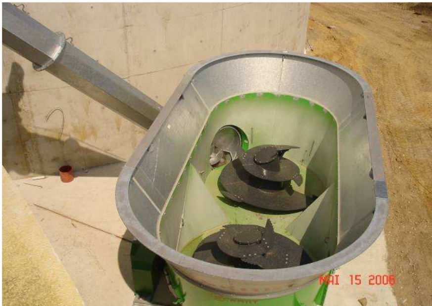
Figure 7.14 Feed-in system for silage (AGRINZ 2006)
