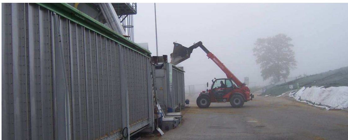
Figure 7.11 Loader feeding maize silage into a container (RUTZ 2008)
